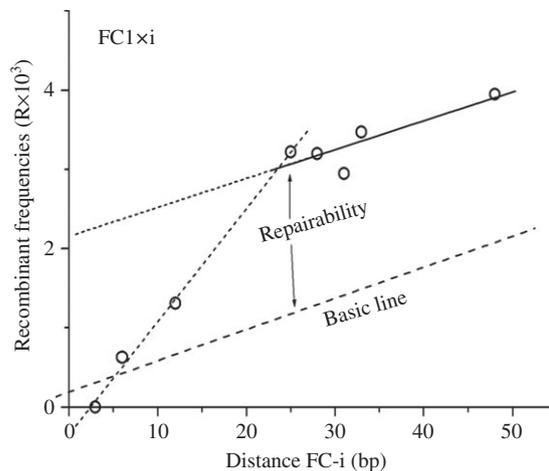
**Figure 3** An example of measuring the repairability value and repair tract length.
