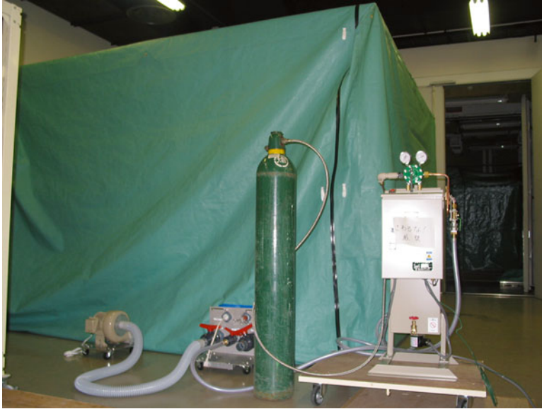
Fig. 2 Carbon dioxide treatment using a fastner bag
