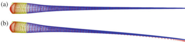
Fig. 18.16 DTU 10 MW RWT modal analysis initial deformation ( blue-yellow ), superposed to the blade geometry reference ( red ) at rated speed . (a) Straight blade. (b) Prebent-precone blade
