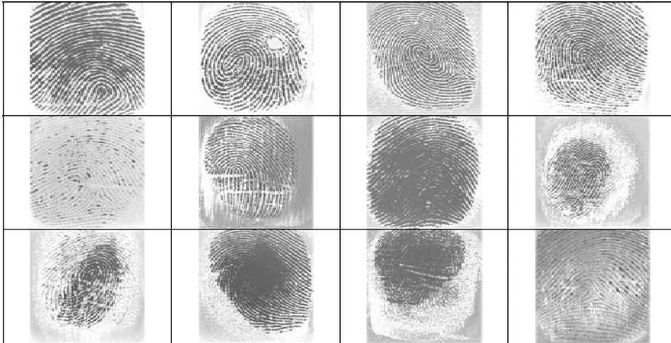
Fig. 6. Images from DB2; all the samples are from different fingers and are ordered by quality (top-left: high quality, bottom-right: low quality).
