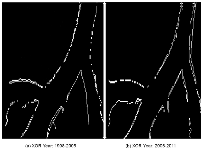
Figure 6 Changes detected by XOR Operation of (a) Im1 (1998) and Im2 (2005) and (b) Im2 (2005) and Im3 (2011).
