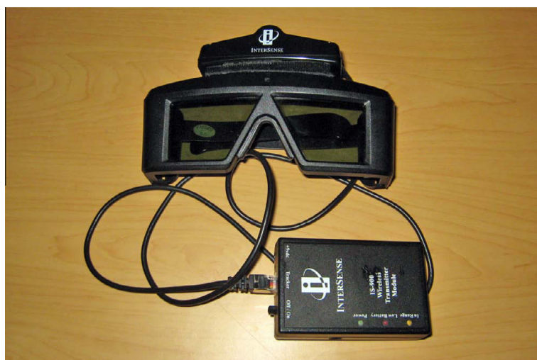
Figure 11 Goggles and head tracker for the CAVE.
