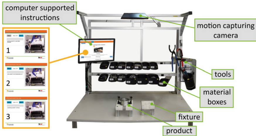
Fig. 7 Smart Assembly Workplace: assembly sequence of bicycle e-hubs is automatically transmitted to the user
