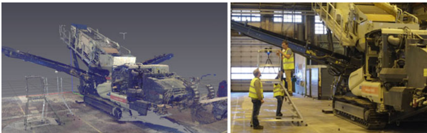
Fig. 3 Laser scanning and generated point cloud representation
