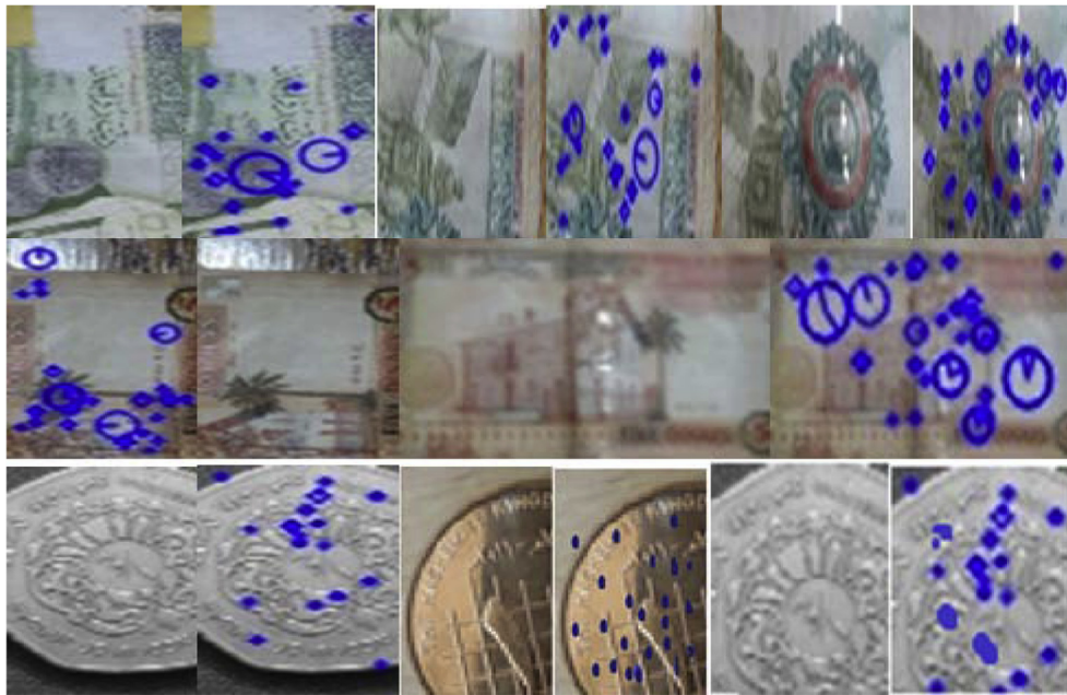
Figure 4 Sample of the tested banknote and the detection of their key-points (color).
