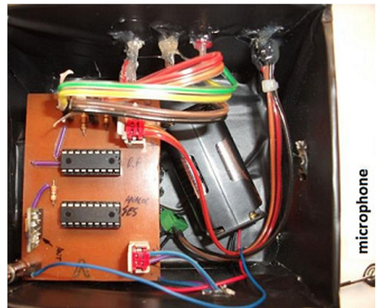
Fig. 7. Microcontroller and voice detection card.
