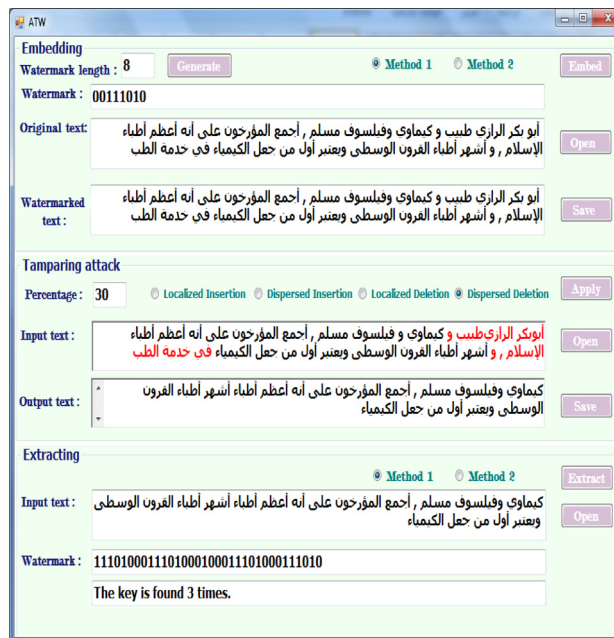
d) Dispersed Deletion attack (deleted words are colored with red in input text).
