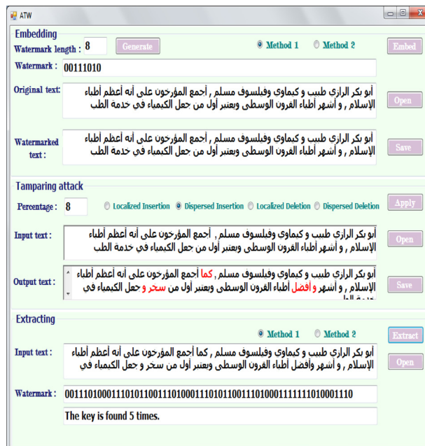
b) Dispersed Insertion attack (inserted words are colored with red in output text).
