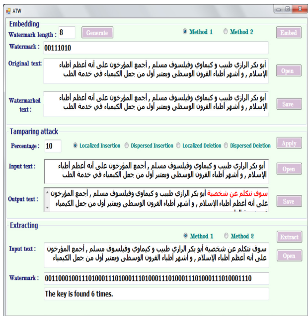
a) Localized Insertion attack (inserted words are colored with red in output text).
