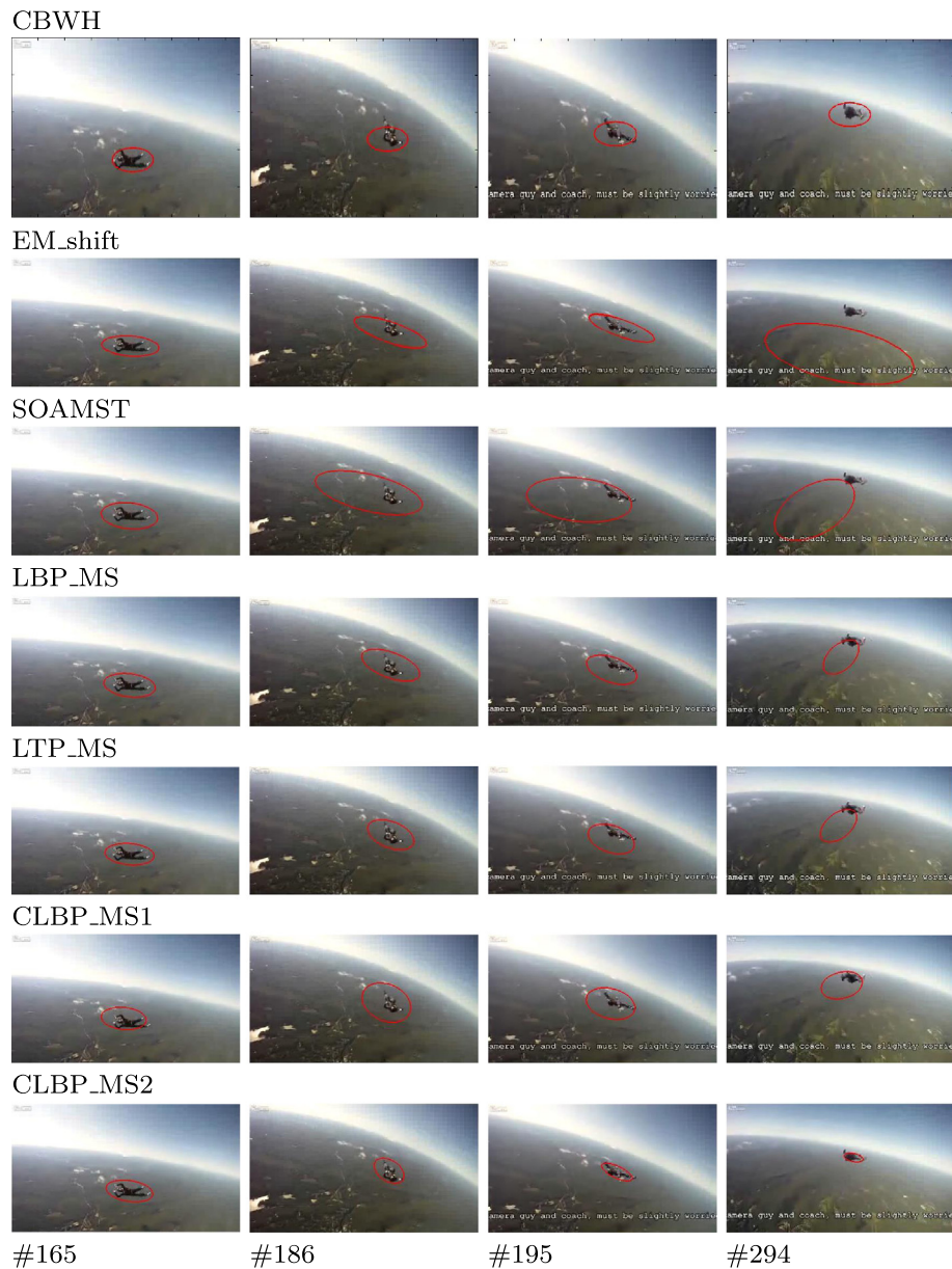
Fig. 9. Tracking results of a parachuting sequence by the target representation models CBWH, EM_shift, SOAMST, LBP_MS, LTP_MS, CLBP_MS1, and CLBP_MS2. Frame 165, 186, 195, and 294 are displayed.
