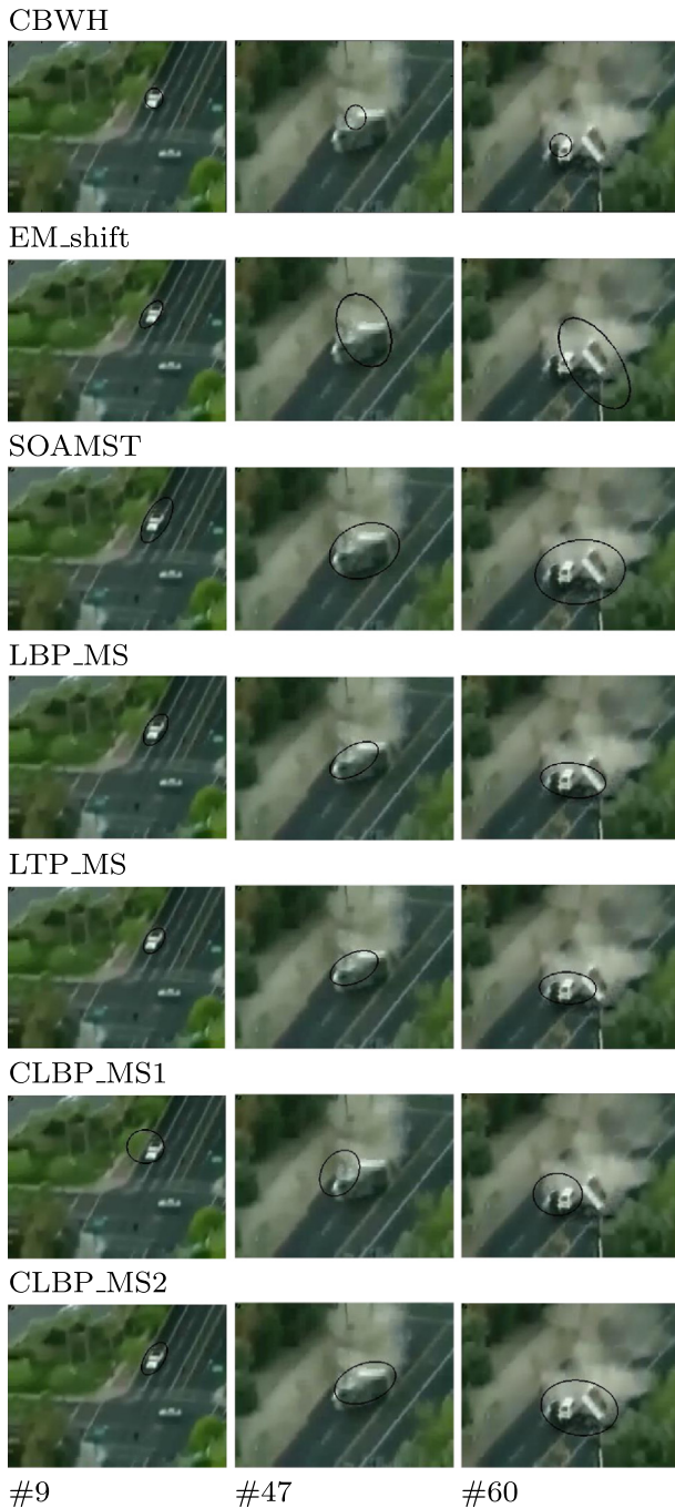
Fig. 7. Tracking results of a white truck sequence by the target representation models CBWH, EM_shift, SOAMST, LBP_MS, LTP_MS, CLBP_MS1, and CLBP_MS2. Frames 9, 47 and 60 are displayed.
